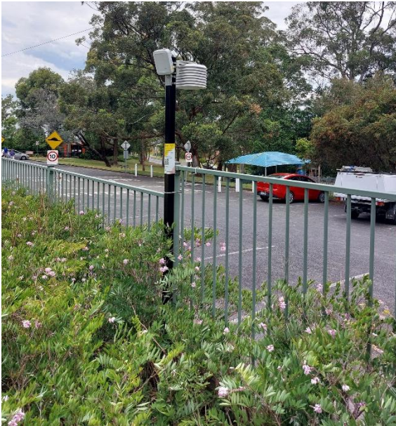
Figure 12. Equipment-facing people counters installed on a pole fastened to the fence near the swings (left) and on a sign pole near the carpark (right).
