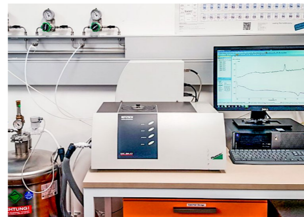
Netzsch DSC (Cold-Stage) 204F1 Phoenix
