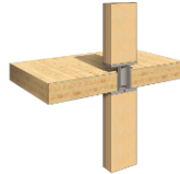
CLT floor slabs with glulam columns and steel connectors
