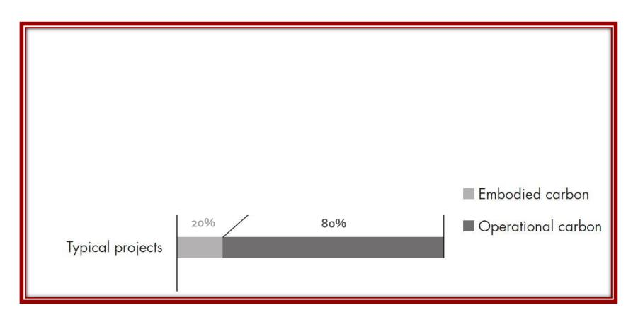
The ratio of embodied carbon to operational carbon during implementation of energy efficient buildings
