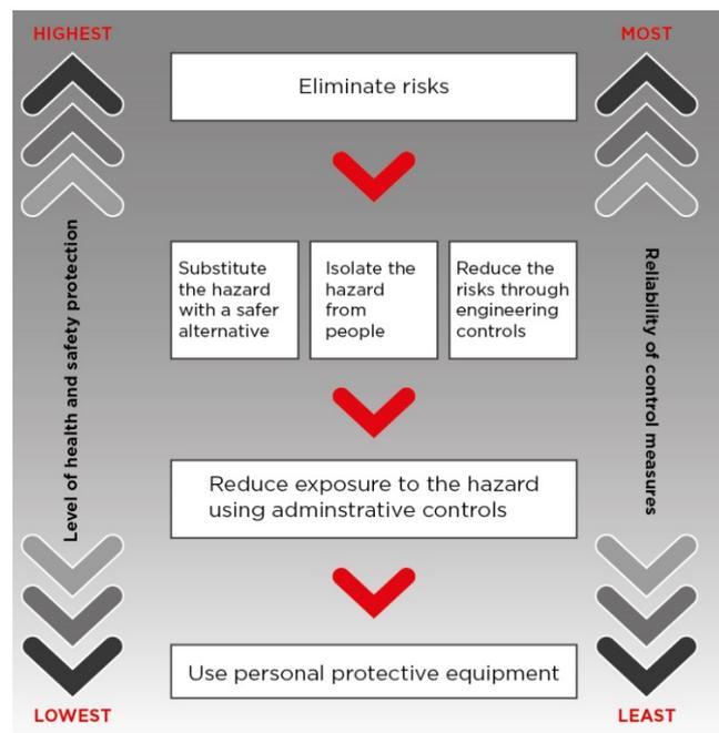
Figure 2 The hierarchy of control measures
