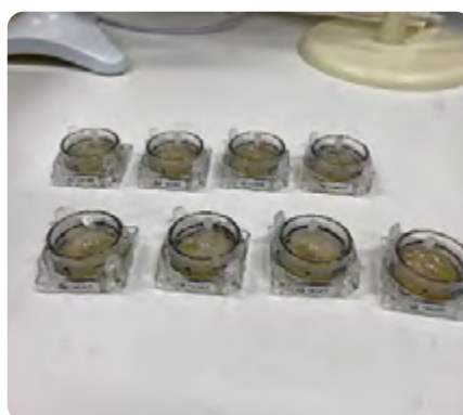
Left: The single-cell RNA sequencing HIVE™ collector devices. Right: The base of HIVE™ collector device sealed with the membrane for further lysis, hybridization and bead recovery processing, followed by later synthesis and amplification steps to generate the sample library, for single-cell RNA sequencing.
