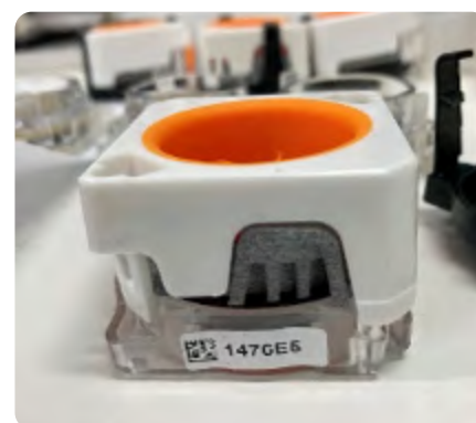
Left: The single-cell RNA sequencing HIVE™ collector devices. Right: The base of HIVE™ collector device sealed with the membrane for further lysis, hybridization and bead recovery processing, followed by later synthesis and amplification steps to generate the sample library, for single-cell RNA sequencing.
