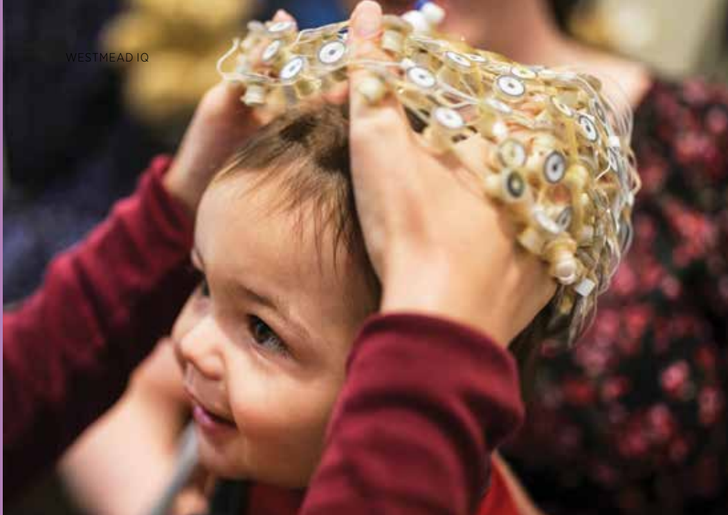
Psychophysiological assessment with continuous measurements using an electroencephalography (EEG) cap in the Westmead BabyLab.
