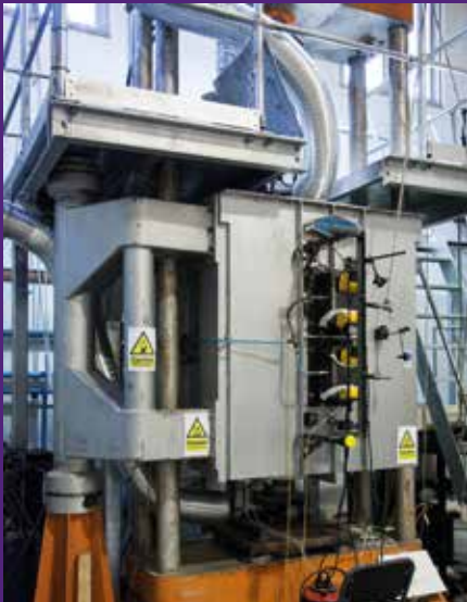
Elevated Temperature Test Rig (Up to 900°C, 200 tonne)
