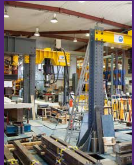
Strong Floor 8m x16m and associated Testing Rigs
