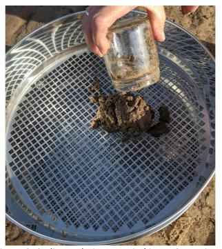
Figure 3: Sediment being emptied into 10mm sieve.
